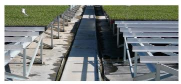
T-rail refers to an aluminum extrusion that is in the shape of an inverted T. They are designed for Styrofoam plug trays that are stiff enough to span between the extrusions. A base of steel bench legs and runners is required to support the trays. T-rail benches are fixed. The trays can be slid from the center aisle of a greenhouse to the sidewall or to one end for pickup and transfer. This system is used for intensive large scale transplant production.
